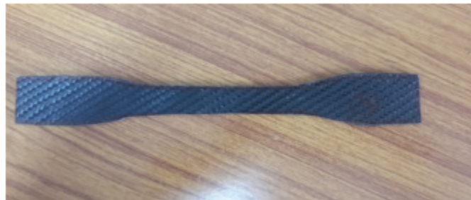
Fig. 7. Specimen wrapping with carbon fibre
