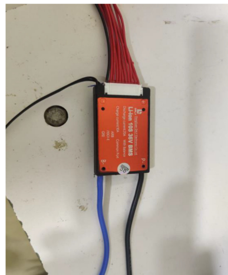
Fig 3.7 Battery management System
