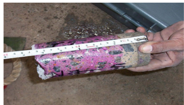
Figure 14: Carbonation Depth measurement Source: Internet
