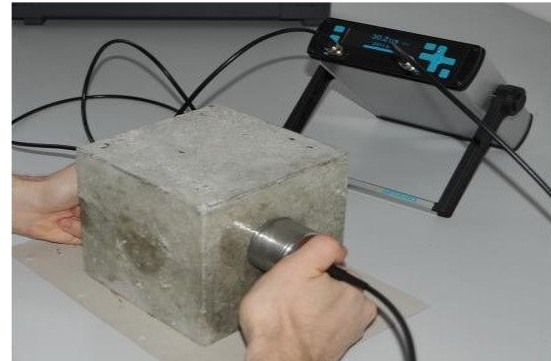
Figure 4: Ultrasonic pulse velocity test Source: Internet
