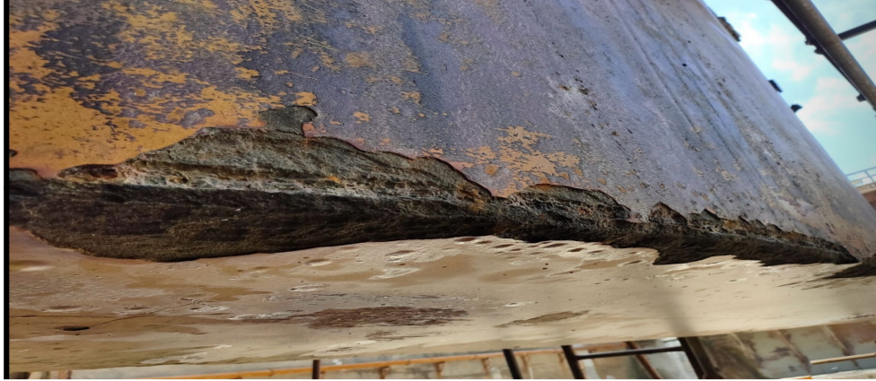
Figure 4 – Cavitation erosion at rudder leading edge.
