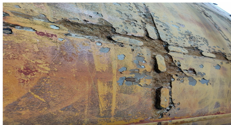
Figure 3 Extensive pitting corrosion and coating delamination on rudder surface.
