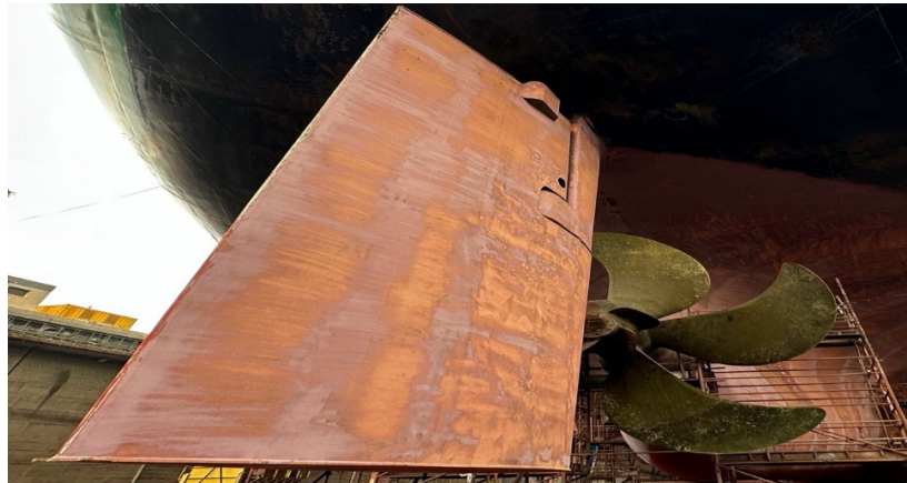
Figure 7 – The LNG carrier rudder and associated assemblies were coated with a glass flake epoxy system, followed by an antifouling coating. The photograph shows the condition of the coating system upon arrival in drydock after 60 months of service. The inspection confirms that the coating remains in good condition, with no visible signs of localized pitting corrosion, cavitation erosion or coating delamination on rudder surface.
