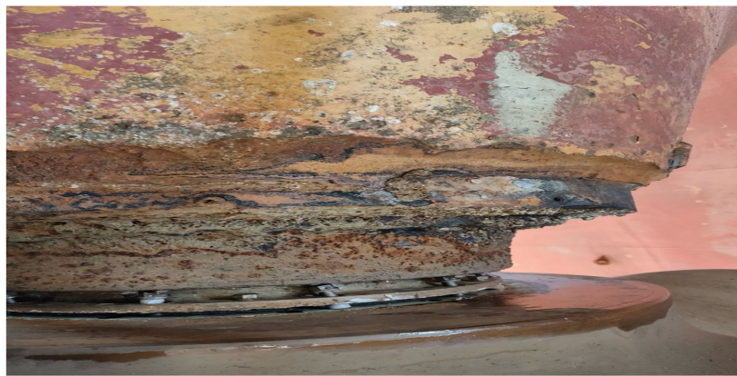
Figure 5 – Microbial corrosion and surface degradation on rudder gear mount.
