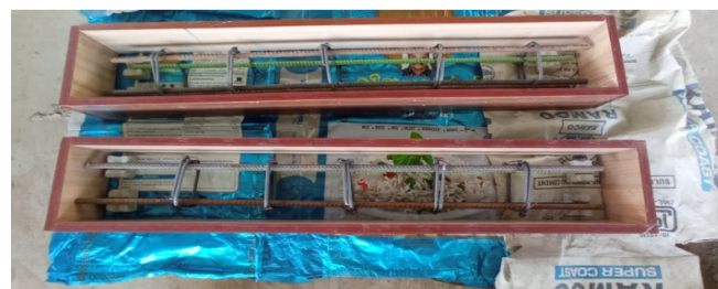
Fig 1: Beam with Reinforcement details.
