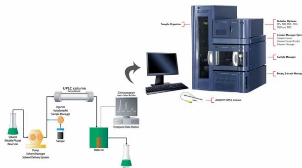
**Fig.No.3: UPLC Instrumentation**
