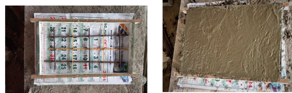
Both steel &amp; GFRP reinforcement Casting of slab
