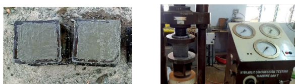
Fig 1 Casting and Compression test on concrete cube
