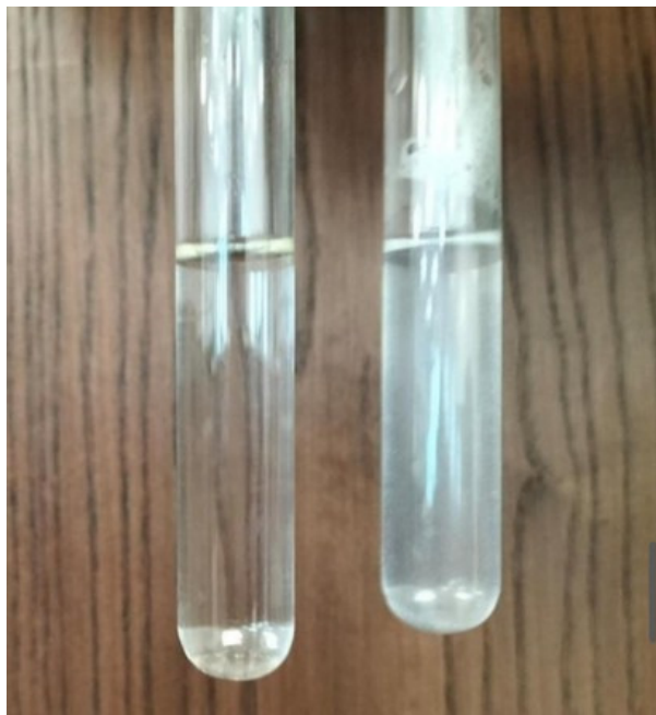
Figure 7:- Comparision Between Purified Water (left test tube) and Initial Greywater(Right test tube)
