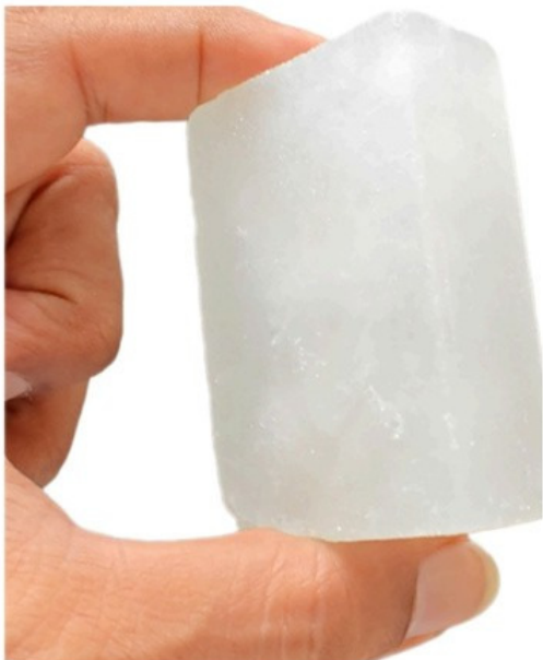
Figure 3:- Solid Alum used to purify water
