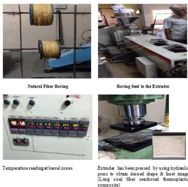
Figure 5 Fabrication of Specimen
