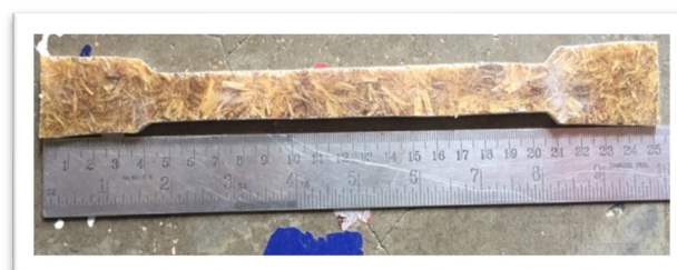
Figure 6 Dog Bone Shape for Tensile Test Specimen
