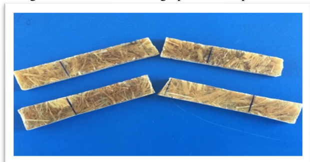
Figure 12 Breakage of Flexural Bending Tested Specimen
