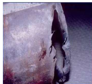
Failure of 14" heater drain extraction line to high pressure heater at Arkansas unit 2, 1986
