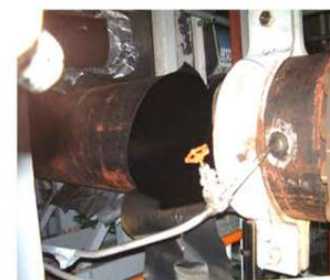
Wall Thickness reduced from 10 to 1.5 mm on Feed-water piping at Mihama unit 3, 2004
