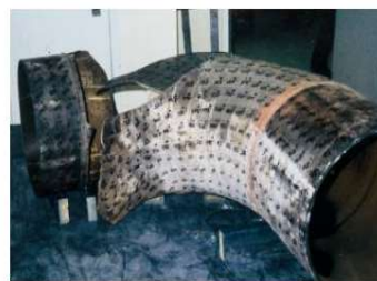
18" elbow wall thickness decreased from 12.7 to 1.5 mm on feed-water pump inlet at Surry, 1986
