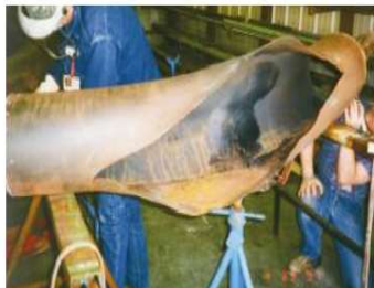
Failure in a high pressure extraction line at Fort Calhoun in 1997
