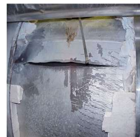
Failure of the Feed-water Heater Point Beach Unit 1, 1999
