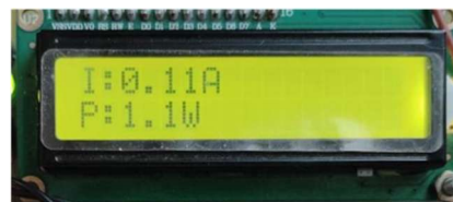
Current and Power Monitoring
