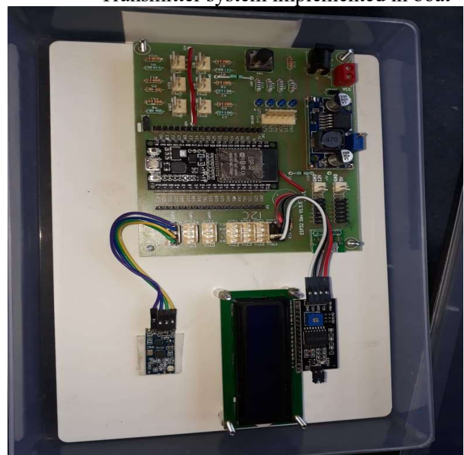
Receiver in base station
