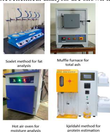
Fig. 2: Instruments used for physicochemical analysis including Soxhlet apparatus, muffle furnace, hot air oven and Kjeldahl apparatus.
