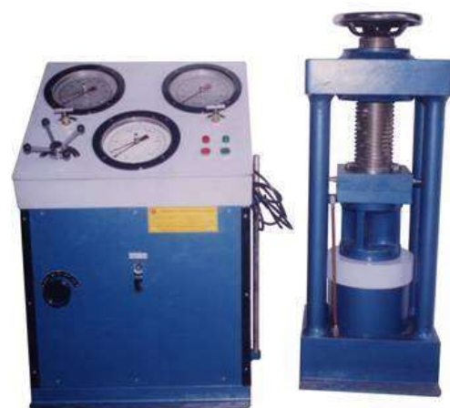
Fig.3. Crushing strength test of aggregate on UTM
