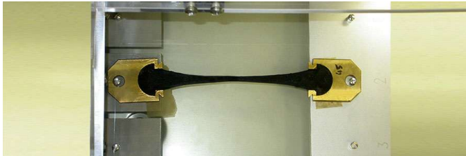
Fig 6. Ductility test on bitumen
