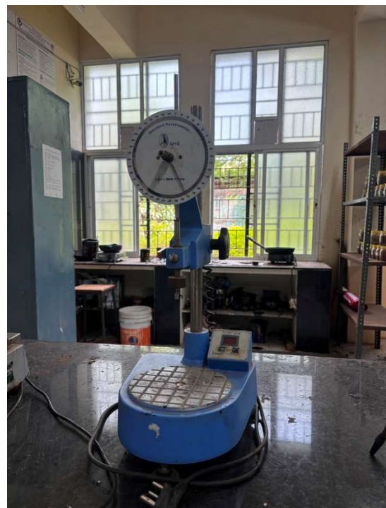
Fig.5. Penetration test of bitumen.
