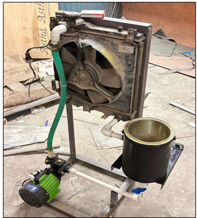
Fig. 3 Photographic representation of the complete experimental system used to conduct research into the use of nanofluids as radiator coolant.
