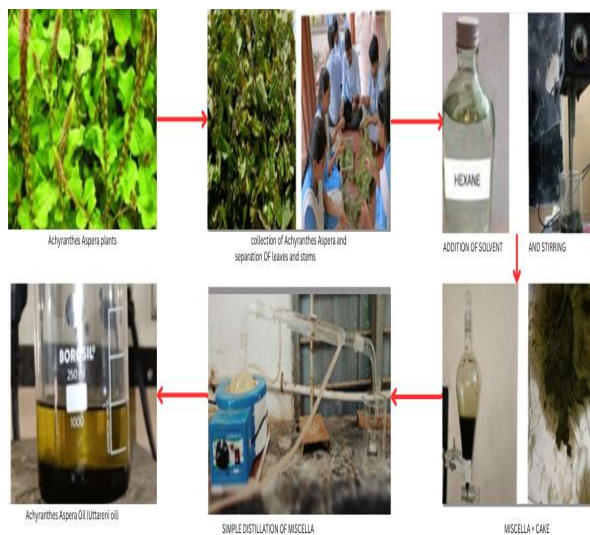
Fig.3 . Flow sheet for extraction of Achyranthes aspera oil
