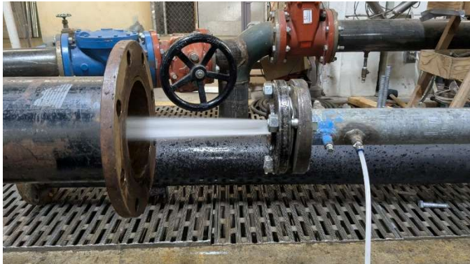
Fig. 5 Image of the atmospheric discharge test configuration with an orifice installed; flow was right to left. The catchment pipe on the left is set a distance away from the test device as to not draw a vacuum on the downstream end of the orifice. The pressure was monitored from the upstream pressure tap.
