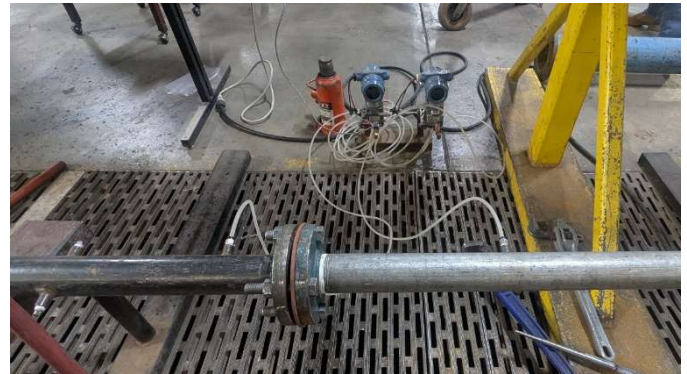
Fig. 3 Image of the test setup with an orifice plate installed; flow is left to right. The pressure taps were connected via plastic tubing to the pressure transducers, where one measured the pressure upstream and one measured the pressure downstream.
