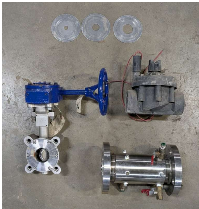
Fig. 2 Image of the valves and meters being tested. Upper: 0.3, 0.5, and 0.7 \beta ratio orifice plates. Left: butterfly valve. Right middle: globe valve. Lower right: Venturi. All valves and meters are for 2-inch diameter pipelines
