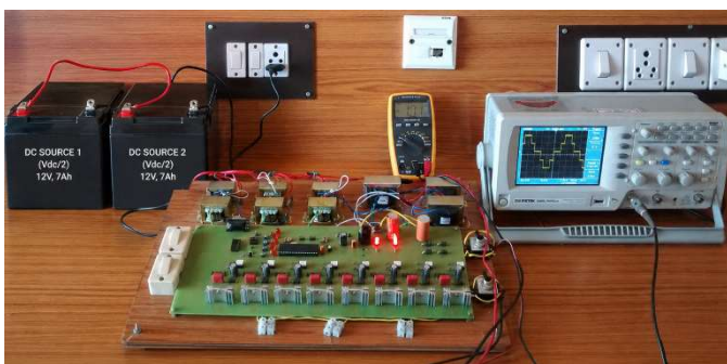
Fig. 4 Experimental setup Modified Cascaded H-Bridge 5-Level Inverter
